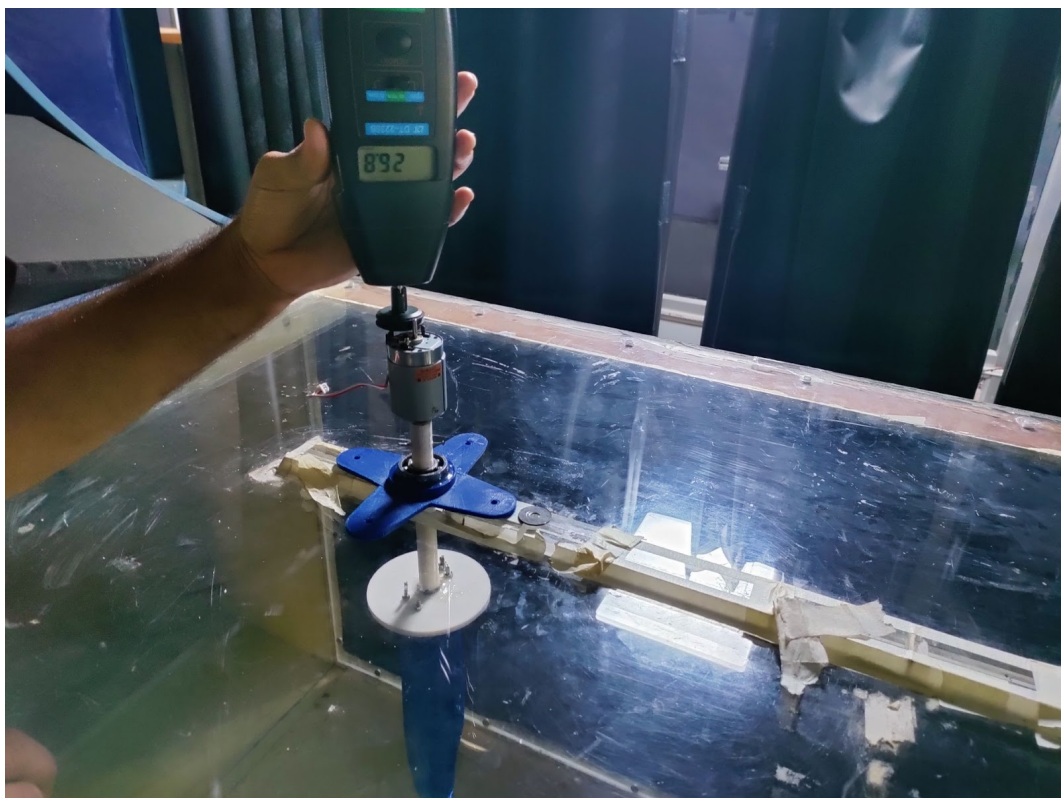
Figure 19. Person measuring turbine rpm using tachometer
