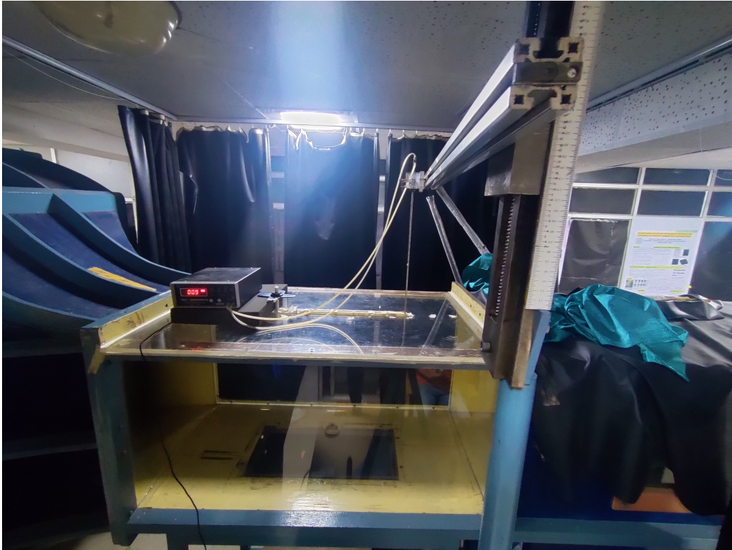
Figure 23. Setup for measuring pitot readings to get velocity profile (Rake)
